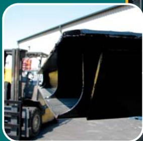
The end of the Weldcoa pallet is shaped like a "C" and cups the center tube of Weldcoa pallet vehicles.
