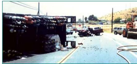
*The picture at far left was taken during the downward restraining force testing. The nearer picture shows how the system performs in an unfortunate accident in which a truck overturned and slid 50 yards. Not a single pallet or cylinder were ejected.*
