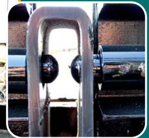
Once engaged, a quick visual inspection can be performed to assure that the pallets are locked in place.
