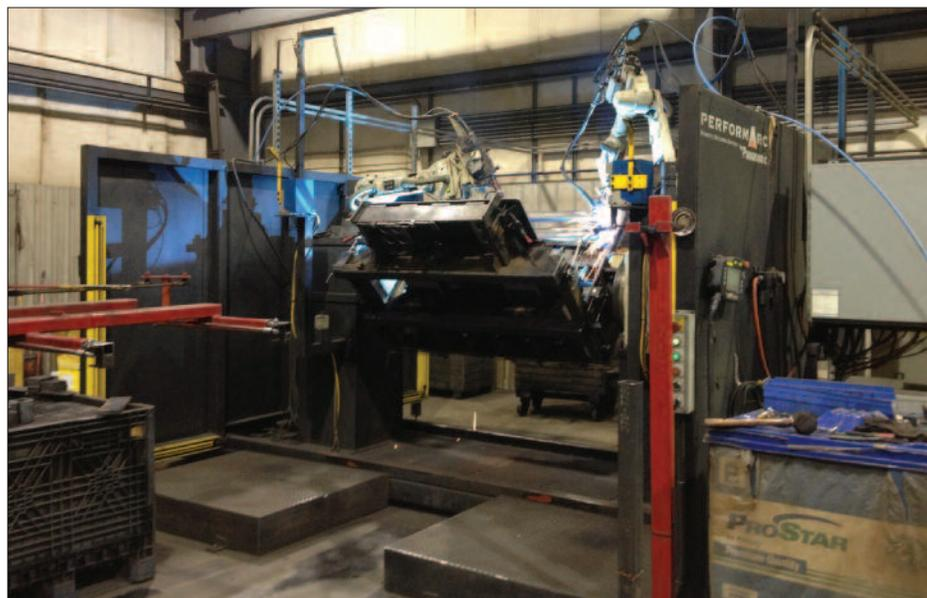
Weldcoa's most recent Panasonic-designed dual arm robotic welding system can produce a complete pallet every eight minutes.
