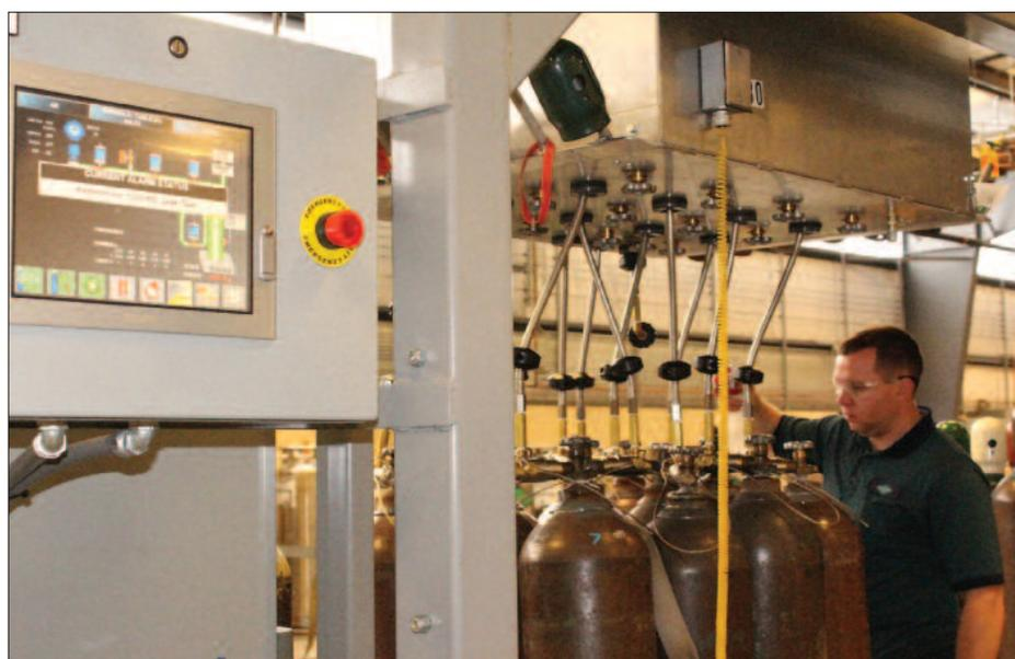
This year, Holston installed a fully automated palletized filling system with 24 cylinder fill bays, 12 moving fill heads, and six operator control touch screens. The entire Fill Island is 82 feet long.
